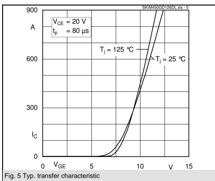
Fig. 5 Typ. transfer characteristic
