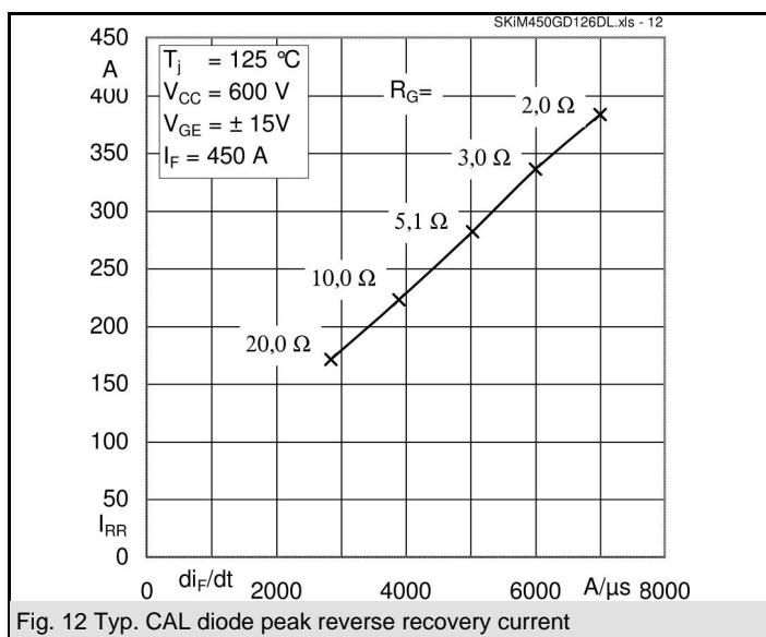
Fig. 12 Typ. CAL diode peak reverse recovery current
