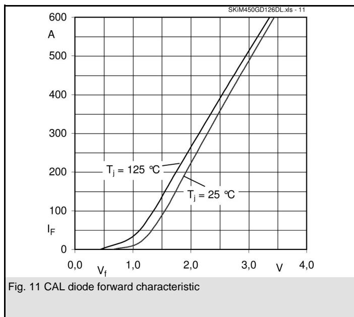
Fig. 11 CAL diode forward characteristic
