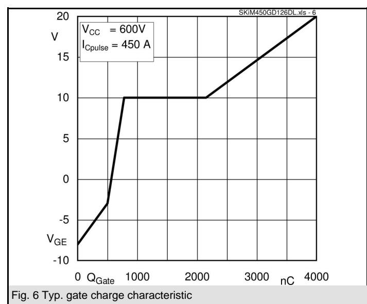
Fig. 6 Typ. gate charge characteristic
