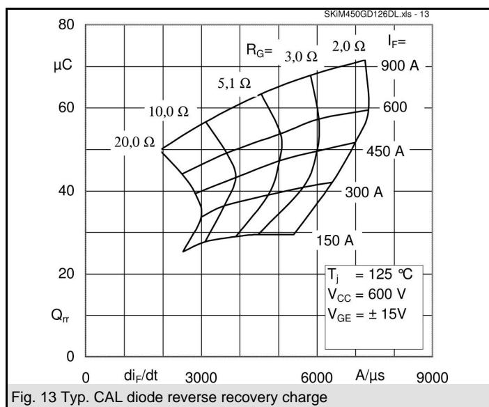
Fig. 13 Typ. CAL diode reverse recovery charge
